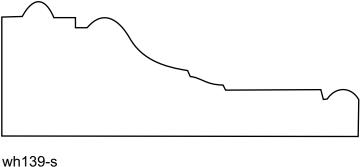
11/16 x 1-5/8 plant-on wood 1-9/16 x 3-3/4 (measured) (casing)
